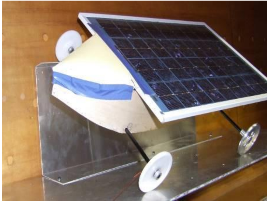
SYNDAL SOUTH 2006 CAR : SIMULATOR AIR DRAG COEFFICIENT 0.0045
