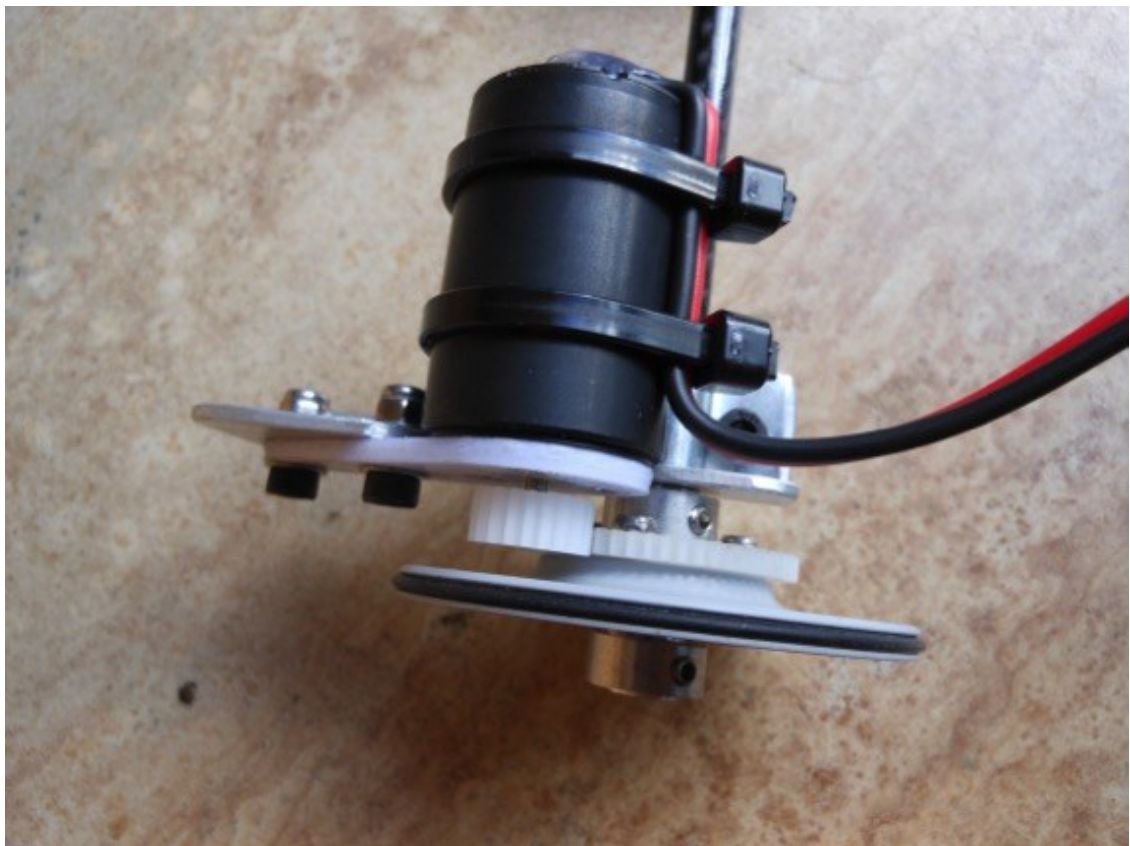
Figure: An example of the completed drive wheel assembly
