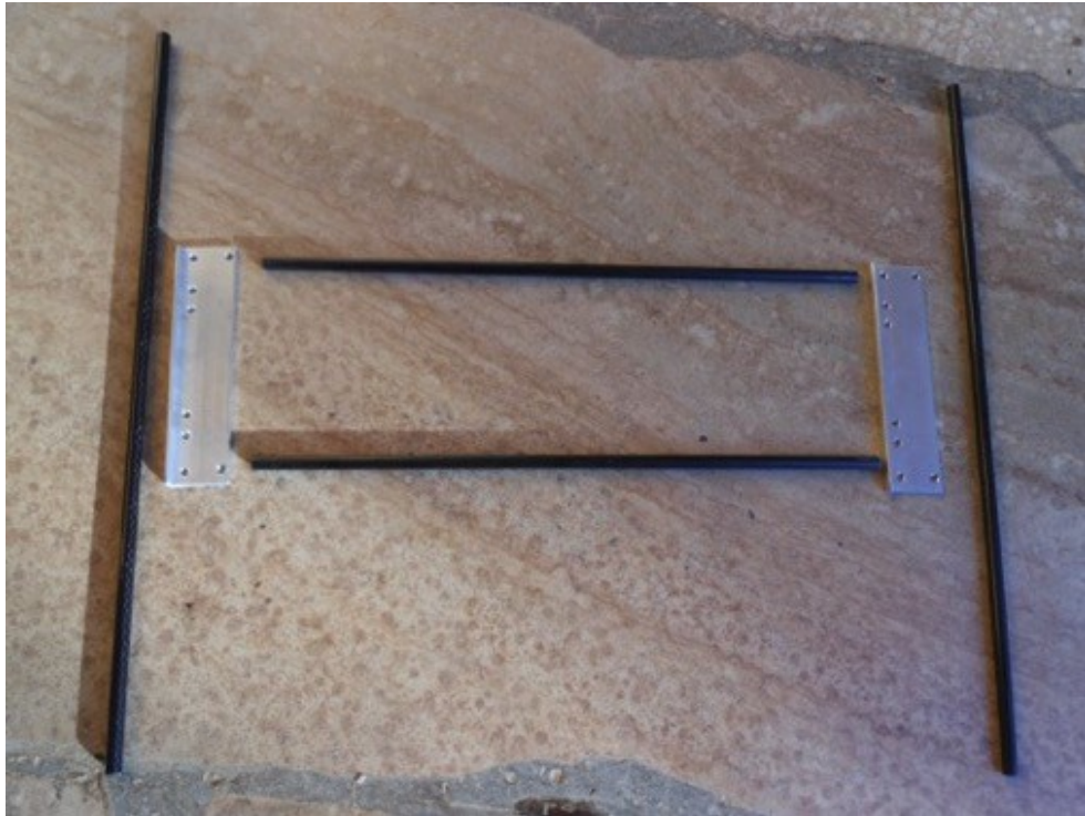
Figure: Frame layout of the 4-wheel kit (front is facing right)
