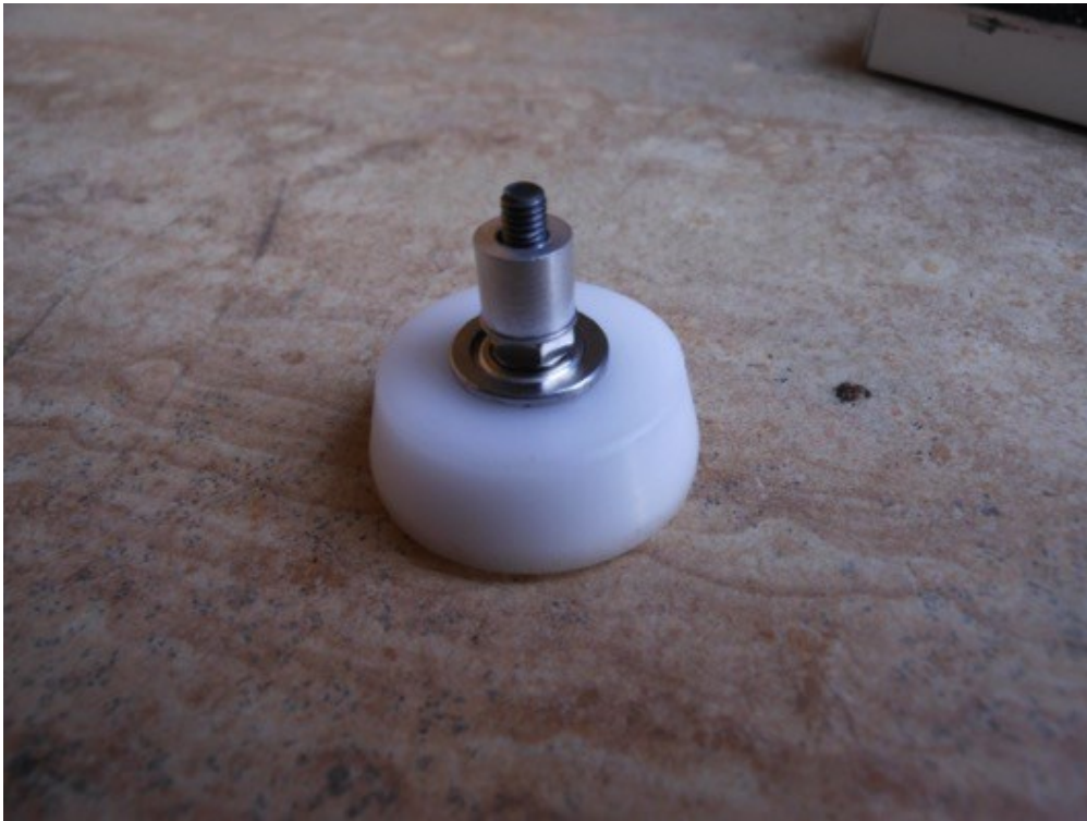
Figure: Roller with nut tightened against bearing followed by a washer and Aluminium spacer
