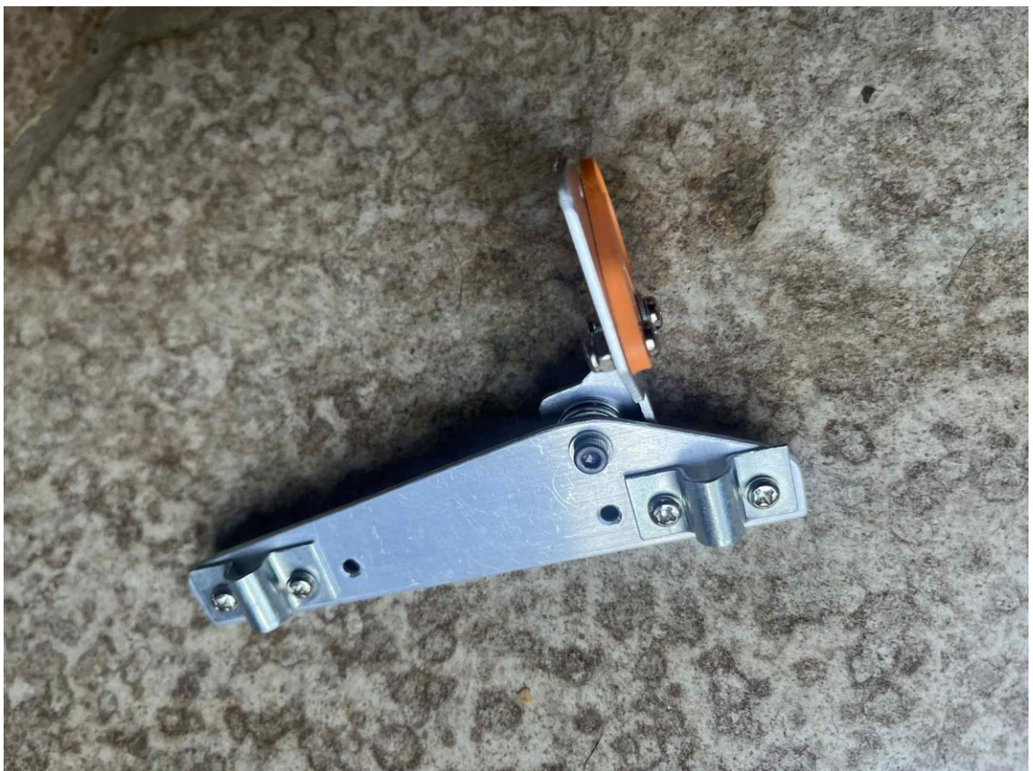
Figure: Rear bracket of the 3-wheeler kit (bottom view)
