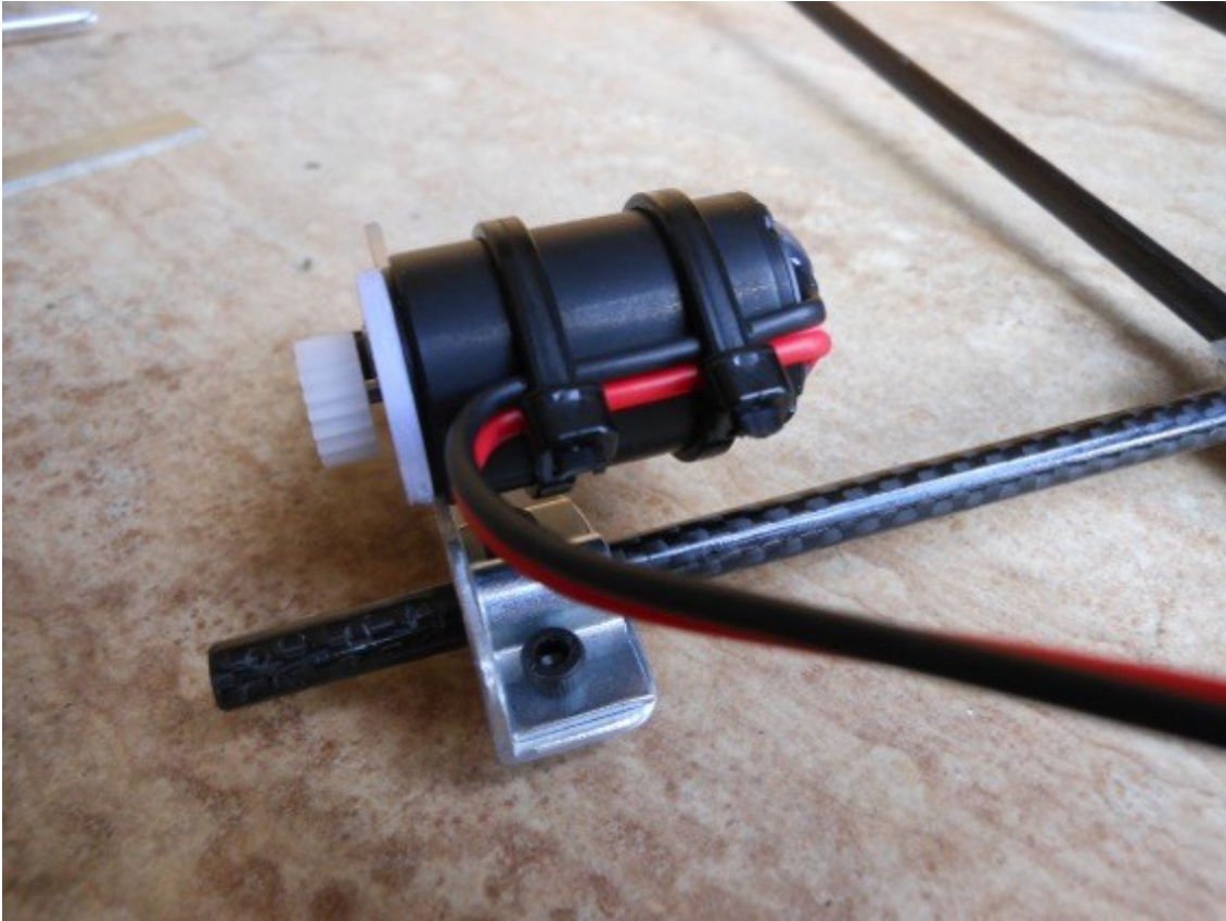
Figure: A small gap should be left between the motor gear and mounting plate
