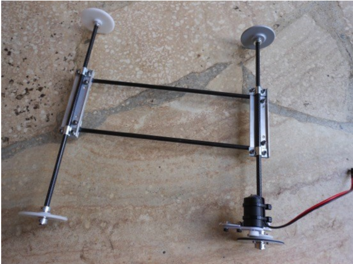
Figure: The 4-wheel chassis with all wheels and motor fitted
