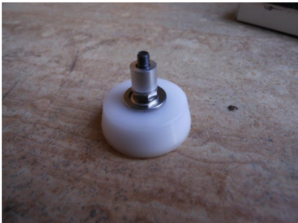
Figure: Each roller has a nut tightened against the bearing followed by a washer and aluminium spacer. This bolt goes through the mounting holes the front and rear brackets.
