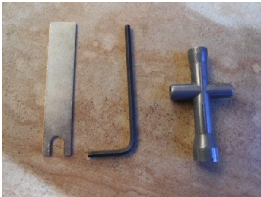
Figure: The kit may include a Multitool Spanner, 2.5mm Allen Key and mini X-Wrench to assist with assembly
