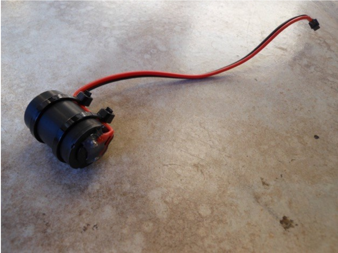
Figure: A Faulhaber motor with wiring and micro deans connector attached
