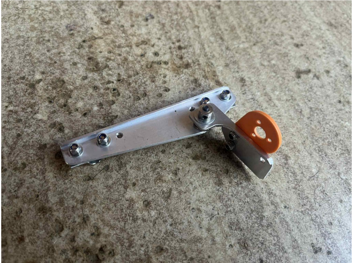
Figure: Rear bracket of the 3-wheeler kit (top view)
