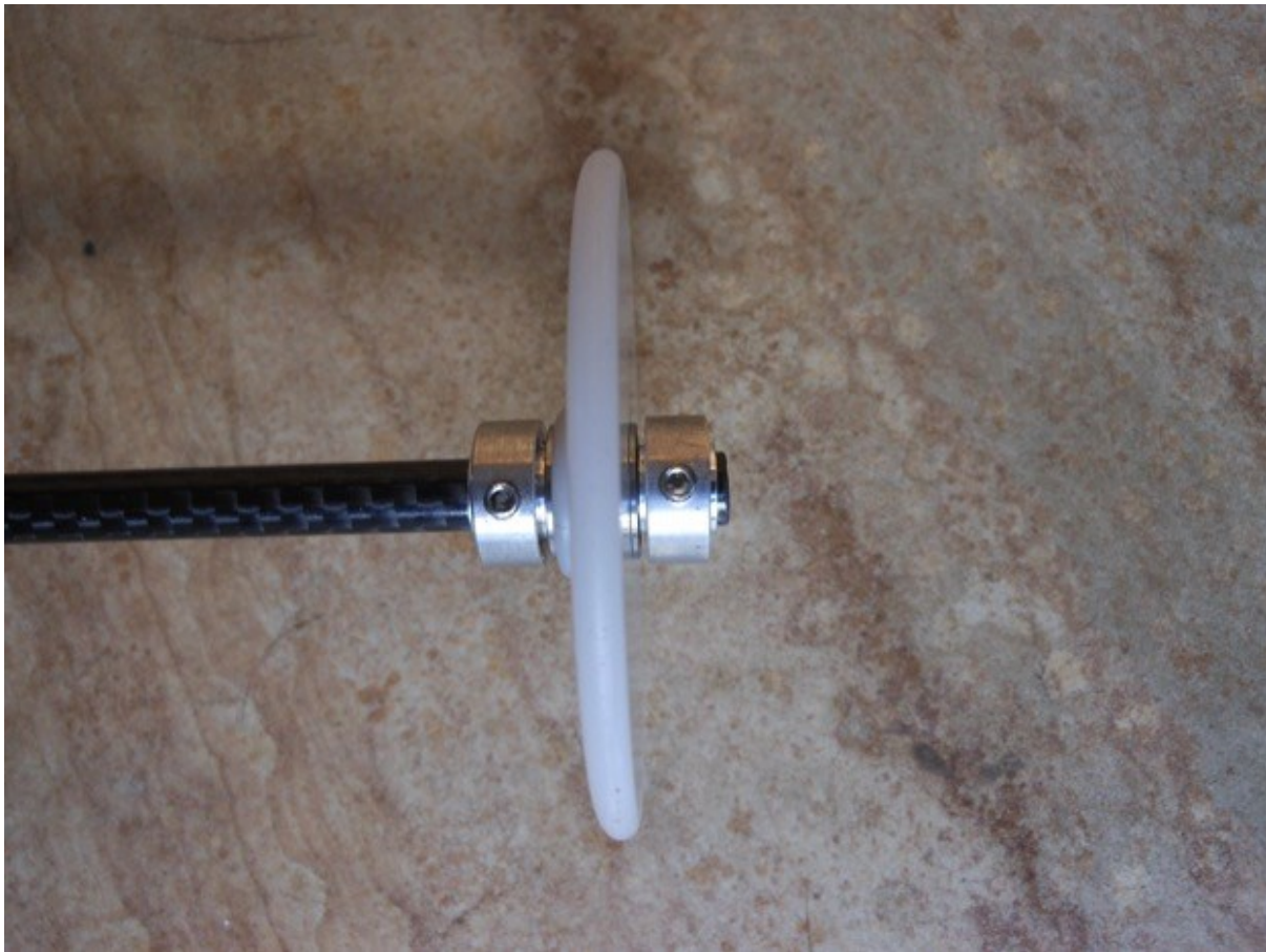
Figure: One of the non-drive wheels fitted between 2 collars
