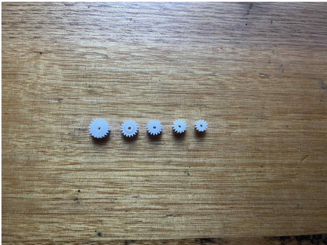
Figure: New kits come with a 20T, 18T, 16T, 14T, 12T and sometimes even 10T gears
