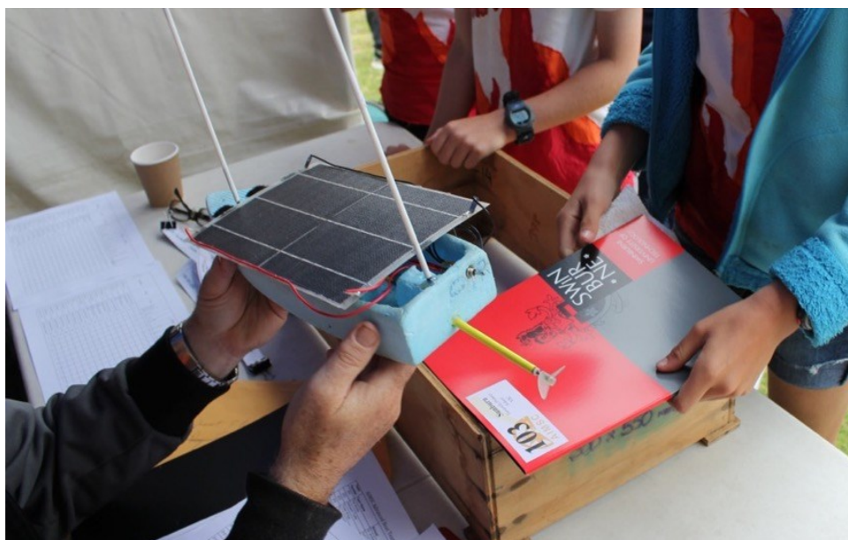
Figure: An example of the yellow tube pushed through the back of a styrofoam hull
