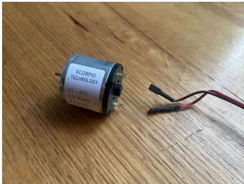
Figure: Any other panels supplied by the TMSC will come with mini spade connectors that fit directly onto the kit motor terminals
