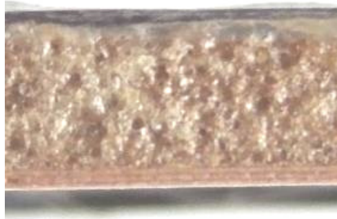
CROSS SECTION OF STRENGTHENED SOLAR PANEL ON TOP CLEGECCELL IN MIDDLE AND PLY ON BOTTOM
