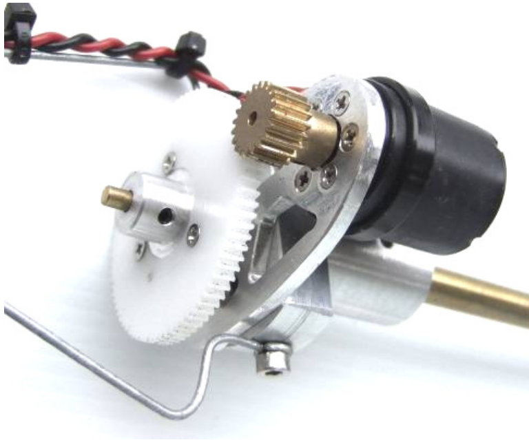
DETAIL OF GEAR REDUCTION TEST SET UP 4:1 RATIO
