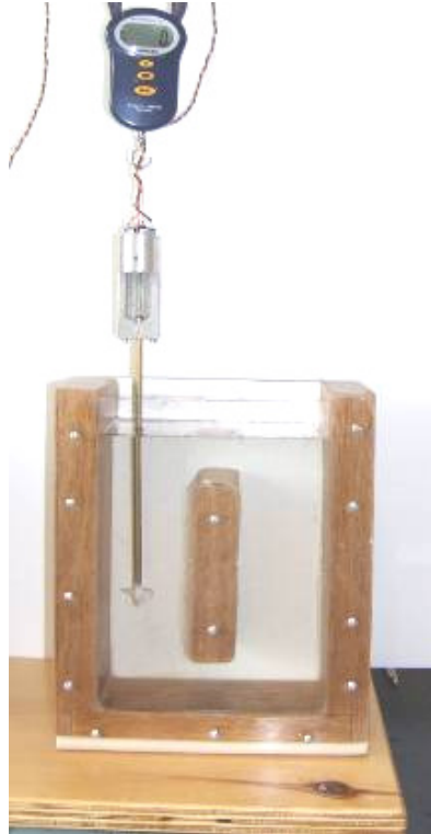
MOTOR AND PROPELLER HANGING FROM BALANCE IN WATER
