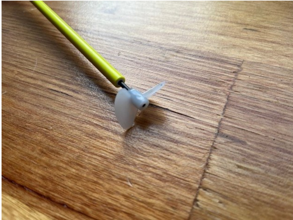
Figure: Each kit is supplied with a 2-bladed nylon propeller
