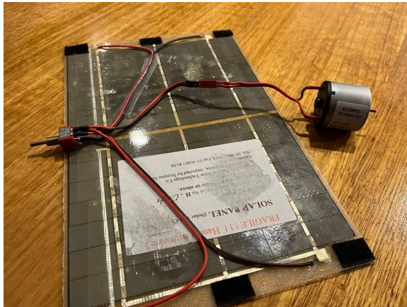
Figure: Event panels include a series-off-parallel switch and plugs directly into all kit motors
