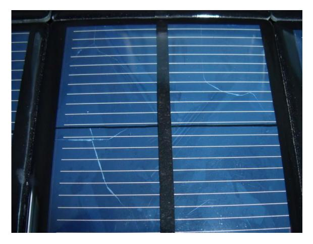
Figure: An example of cell cracking in an Engelec module.
