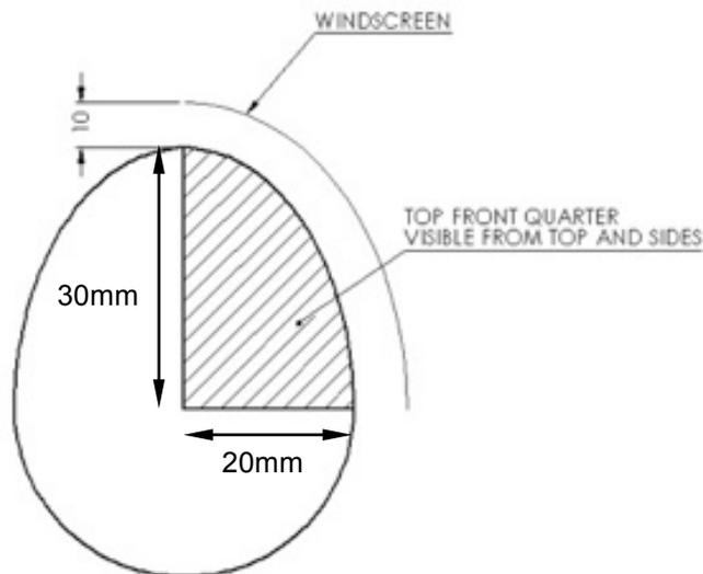
Figure 4 – Egg Driver (all dimensions in mm)
