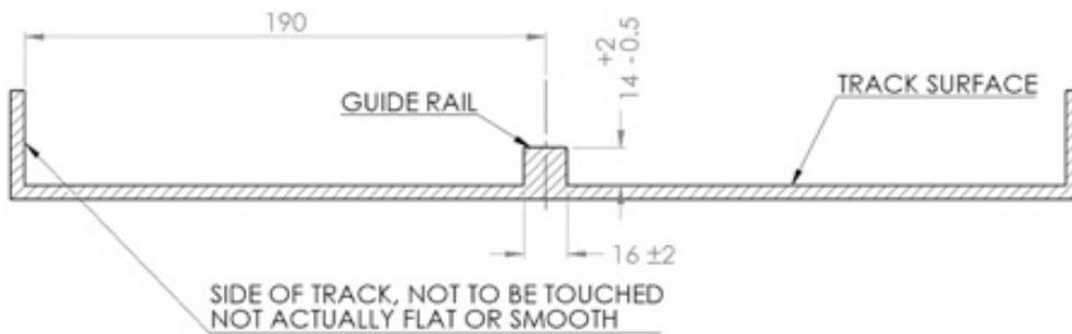
Figure 3 – Track Cross Section (all dimensions in mm)
