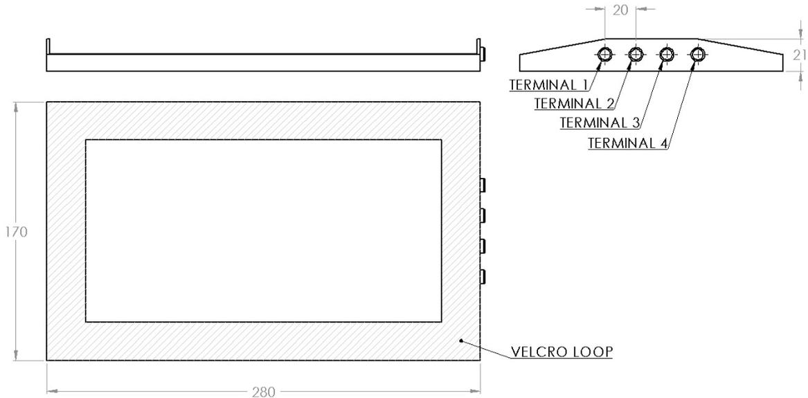
Figure 1 – Competition Array Dimensions (all dimensions in mm)
